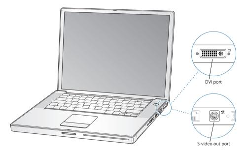
When an external monitor or television is connected, you can either have the same image appear on both the internal display and the external monitor (known as *video-mirroring*) or use the external monitor to extend the size of the Mac OS desktop (known as *dual-display mode*). By default, your PowerBook starts up in dual-display mode. Press the F7 (日) key to switch between dual-display and video-mirroring modes.
